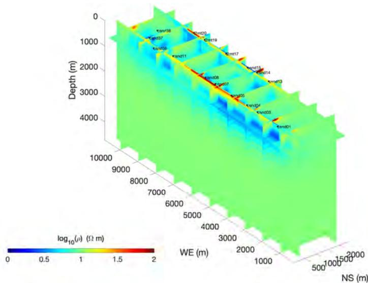
Example of 3D MT inverted data & resistivity model of complex data along two parallel profiles
