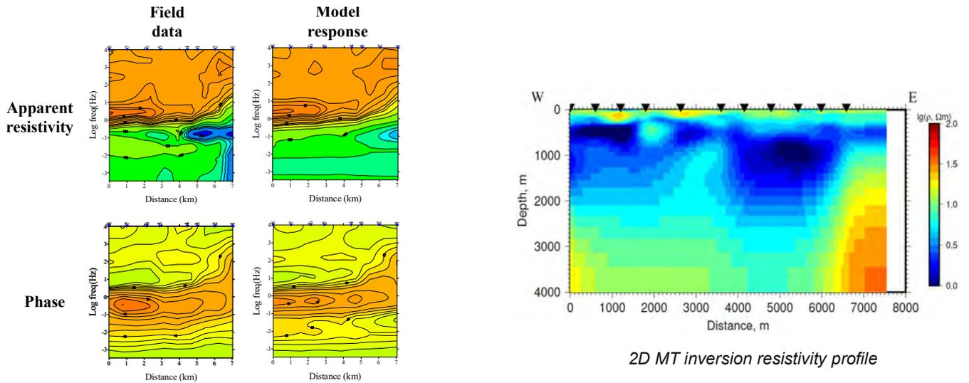
Apparent resistivity (top) and phase (bottom) for acquired field data (left) and 2D MT inverted model (right)
